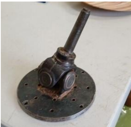
Rob McGregor brought a off-centre camphor laurel bowl he is working on and the off-center chuck he made from a car universal joint and driven with a morse taper.
