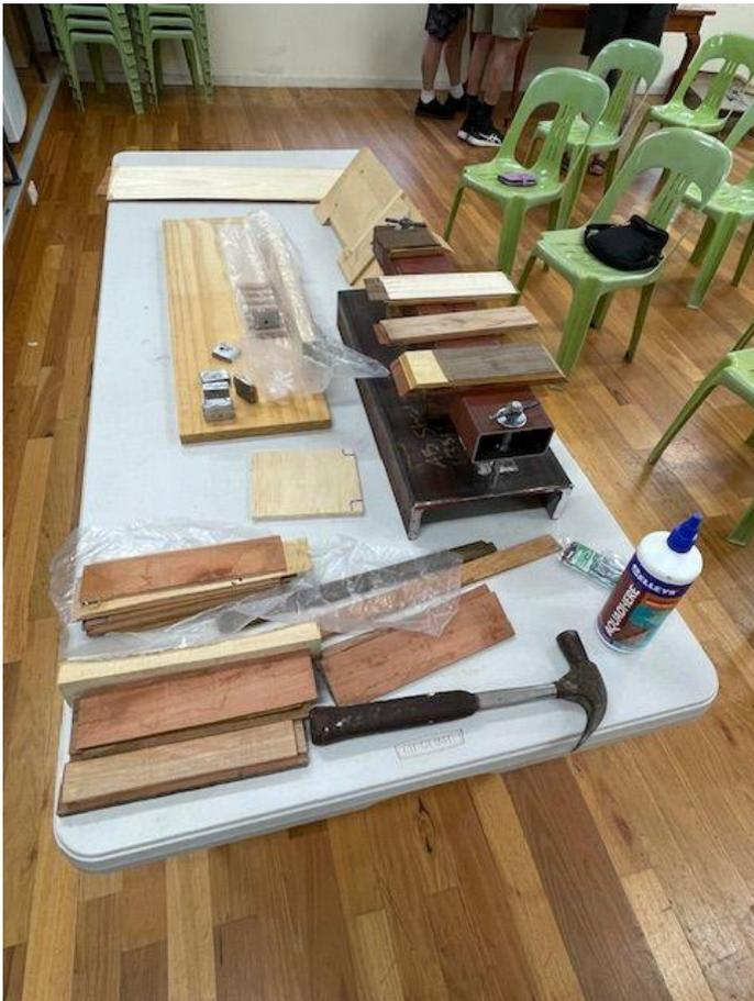
Laminated blocks prepared for slices using jig and bandsaw/dropsaw
