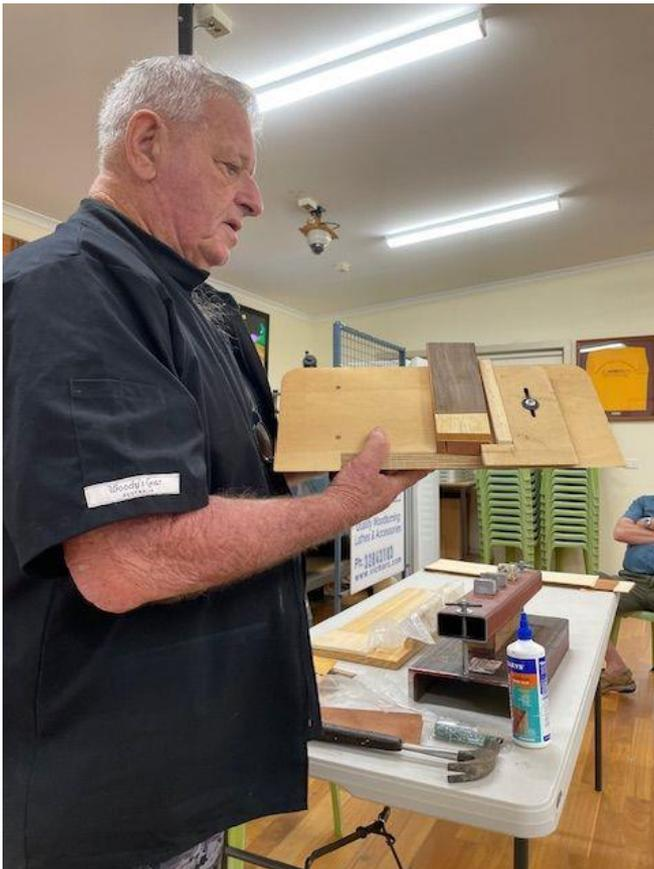
Ken showing the jig and placement of block for cutting
