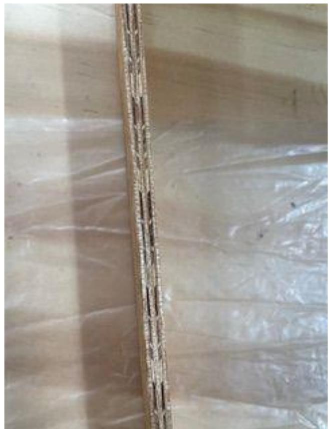
Ribbon prepared for final slicing to form a flexible band
