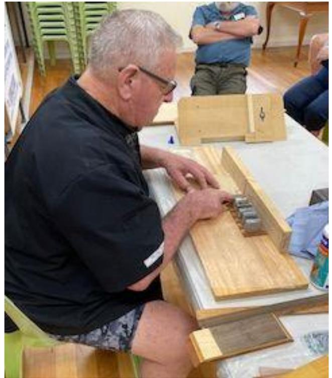
Ken showing slices lined up and glue lines weighted with metal weights
