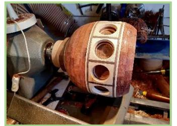
Joining the top and bottom together is aided by this live centre which has a No 2 Morse Taper for the live centre and a thread the same of my lathe spindle so that the face plate can be screwed on making for the whole piece to be rotated.
