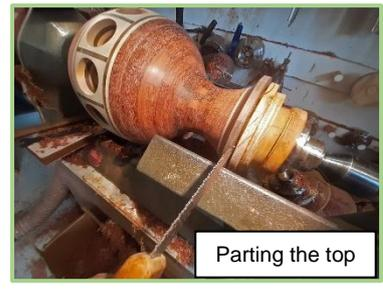
Due to the size the vase was supported with a 3 Point Steady Rest Pro
