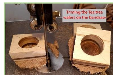
Next the pieces are cut at 15 degrees on each side on the bandsaw and lightly sanded so the pieces will come together as a circle.
