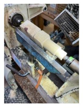
The scene was then set for V-cuts, and the joys of making the sides even. Our V-cuts then became the first stage of cutting beads with the skew.
