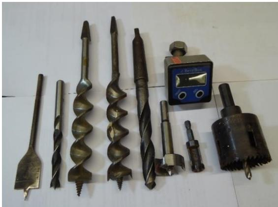
L to R. Spade bit, Brad Point. Auger, Clean cutter Auger, HSS with morse taper, Forstner, Plug cutter, Hole saw, Bevel box.
