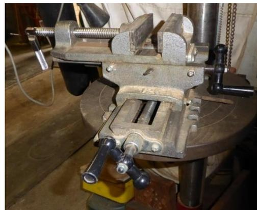
He demonstrated how to cut a slot in timber using a milling cutter, using the Compound Vice.
