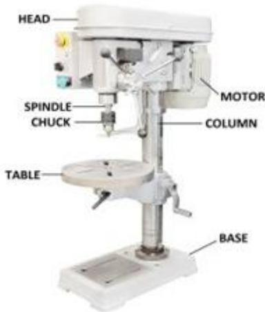
He explained what the various components do and what you can do with them. He covered safety issues, e.g. don't wear gloves, and drilling speeds. Rob discussed issues relating to drilling steel and timber. He discussed the need to use a sacrificial piece of timber between the timber work piece and the table. This prevents tear-out of the timber as the drill comes out of the work piece.
