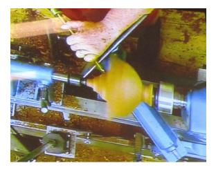
And then, **BANG!!!** The spigot sheared off and the blank hit John in the face!!! Fortunately, he was wearing a very strong full faceshield and neither John or the faceshield suffered any physical damage. The demo blank is shown below.
