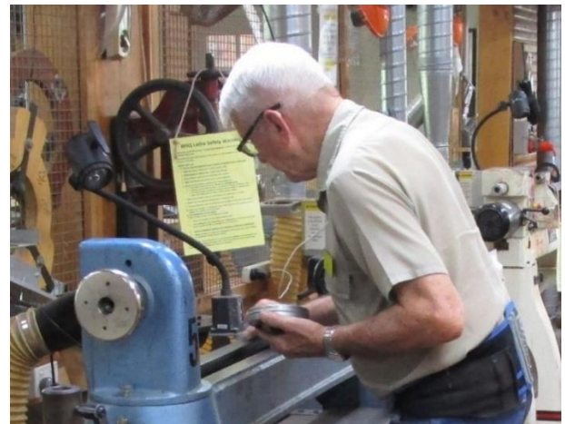
Reg Lubricates the Lathe Bed
