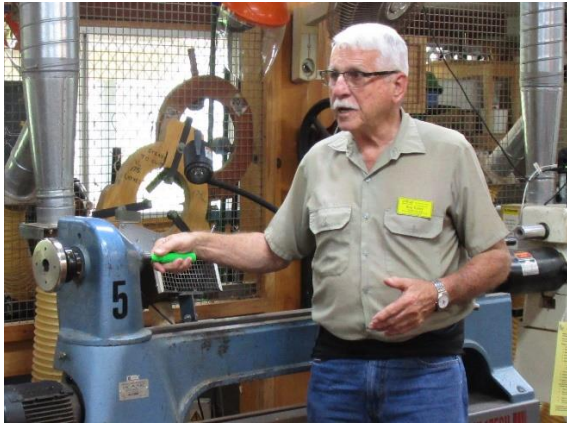
Reg Cleans the Headstock Morse Taper
