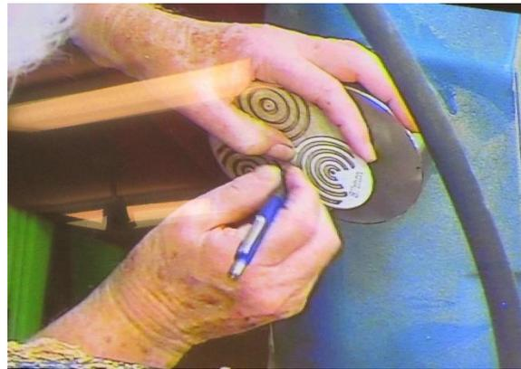
Gary had made the cutting chisel at home using a square section of HSS. The cutting tip is 2.5 mm wide. It has a depth stop with a screw adjustment. Used in conjunction with the flat top toolrest this chisel helps to achieve a square on position for cutting, and depth control to 3 mm.
