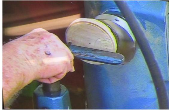
He adjusted the eccentric chuck to a 30 mm offset and marked the centre. He marked 4 lines to be cut using a template as a guide. Gary made a series of light cuts along the marked lines. When the 4 cuts had been made he used the lathe's indexing system to rotate the chuck 120 degrees. He repeated the previous process another 2 times. The marking of the last grouping is shown below.
