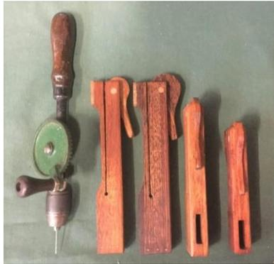
flea market. This hand drill accepts 1mm shaft drill bits. Most electric drills and drill presses won't hold so small a bit. I knew it would come in handy one day. The timber used needs to be at least 5mm thick otherwise the tips protrude and require further attention.
