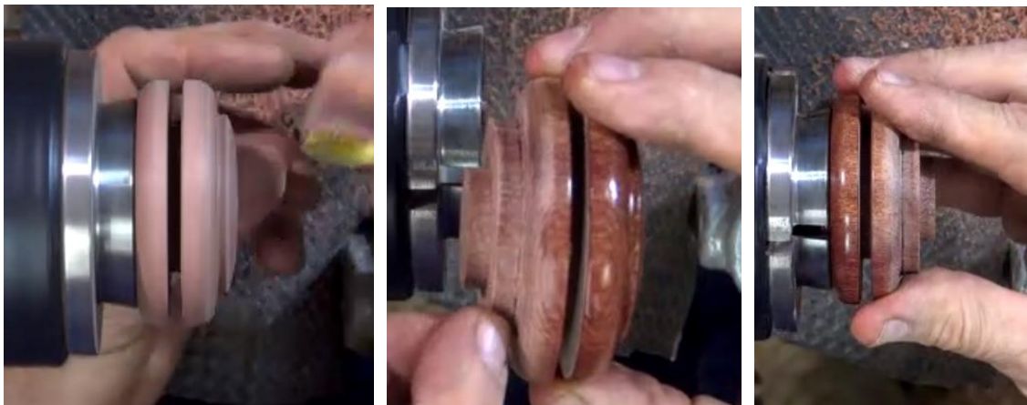
Sanding and finishing the first face of the yo-yo before reversing in the chuck.
