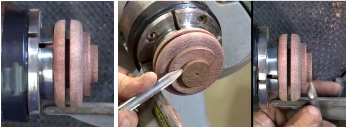
The yo-yo mounted in the chuck for shaping the first side. The composite photo on the right is from a single screen shot, i.e. the images are simultaneous. Note Theo's preferred grip with left index finger curled around behind the tool rest for extra control of the spindle gouge
