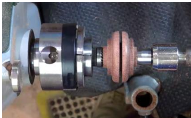
The blank held between centres showing the square spigot either side and the beginning of the central groove. Note the black rubber mat over the bed and banjo, allowing viewers to see the work more clearly. Note also the black electrician's tape around the chuck jaws, which prevents them damaging Theo's knuckles as they spin around.
