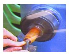
The next stage involved sanding, first with sandpaper – 240g, 320g, 400g and 1200g; followed by micro mesh – 1500g, 1800g, 2400g, 3200g, 3600, 4000g, 6000g, 8000g, 12000g, and 20000g. These involved short, gentle touches. Brian then applied a dot of Shellawax using his finger and a polishing rag.
