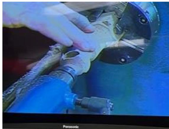
Once again a roughing gouge was used to turn the initial shape, with the spindle gouge then used to refine and size the handle. A small round nose scraper was used to refine the end and sandpaper to deal with the tearing out around the hole.
