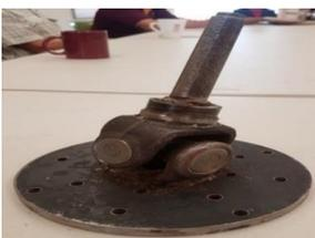
Rob's last entrant was a face plate mounted on an EH Holden universal and morse taper. Very handy for adjusting odd shaped blanks to get the most out of the wood or to set the blank up to keep a feature in the bowl. Mount the
